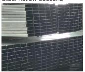
Steel hollow sections are square or rectangular shaped steel pipes. They are typically used where aesthetics are important, such as in furniture and construction of structures. Further, steel hollow sections are also used for lightweight industrial structures and hand railings for construction.
